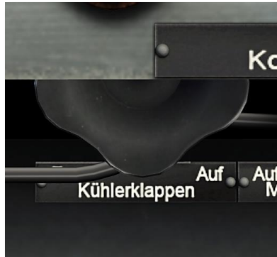
Figure 57: Manual radiator flap control
