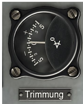
Figure 79: Horizontal stabilizer trim indicator
