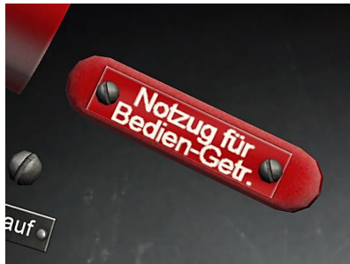
Figure 60: MBG emergency mode handle
