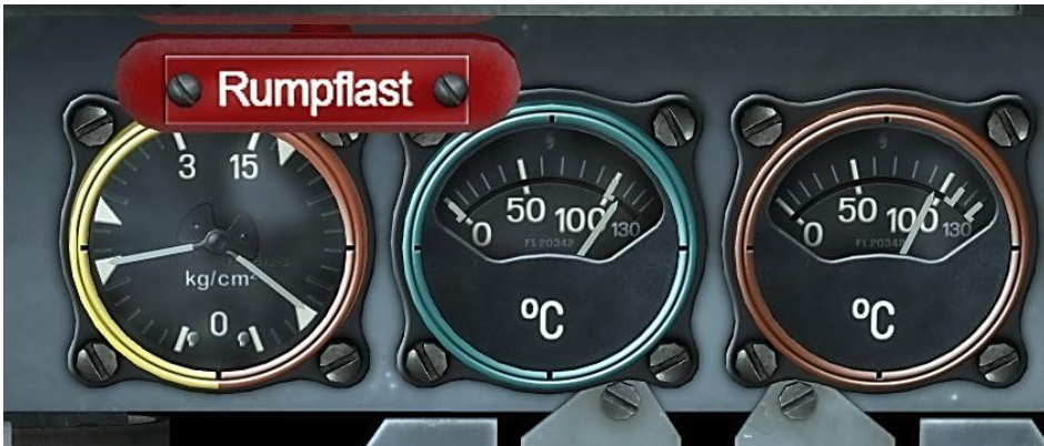
Figure 26: Fuel and oil pressure, coolant temperature and oil temperature gauges
