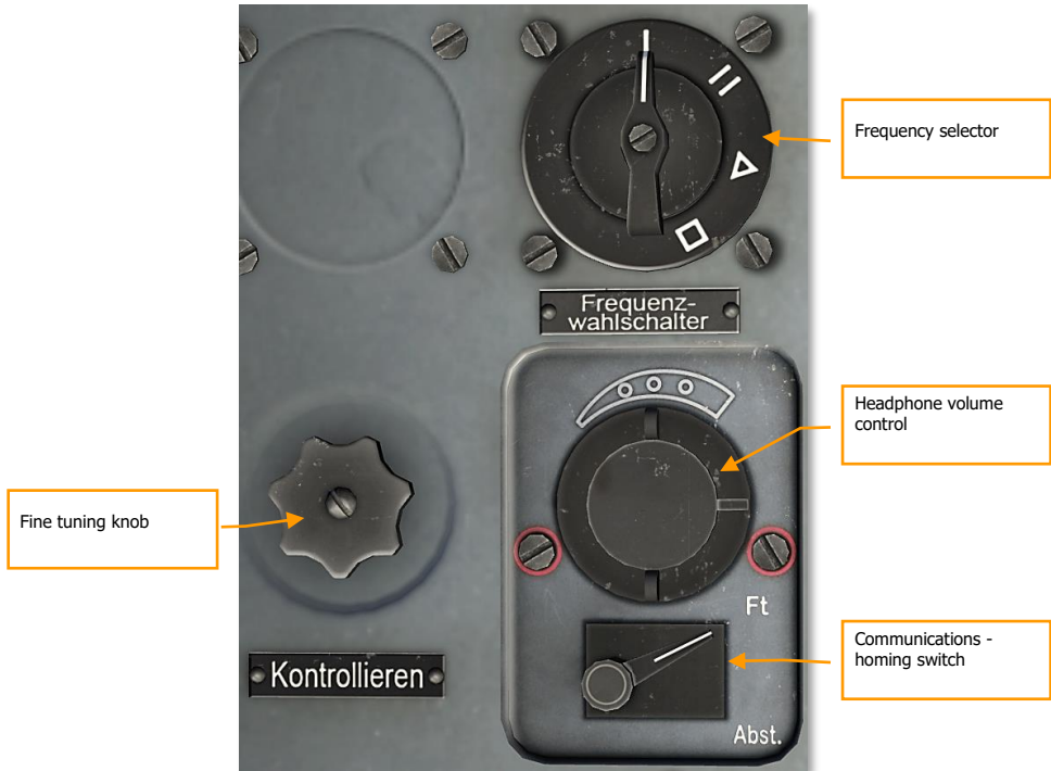
Figure 81: FuG 16ZY controls
