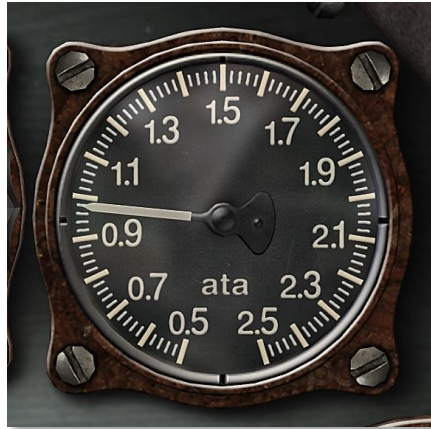
Figure 54: Supercharger pressure gauge
