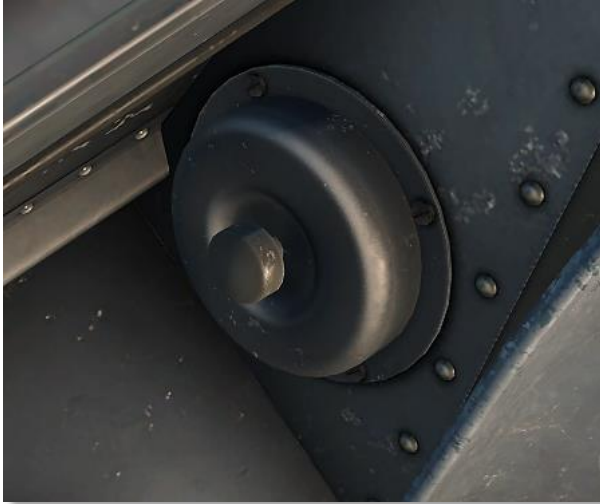
Figure 71: Oxygen emergency knob
