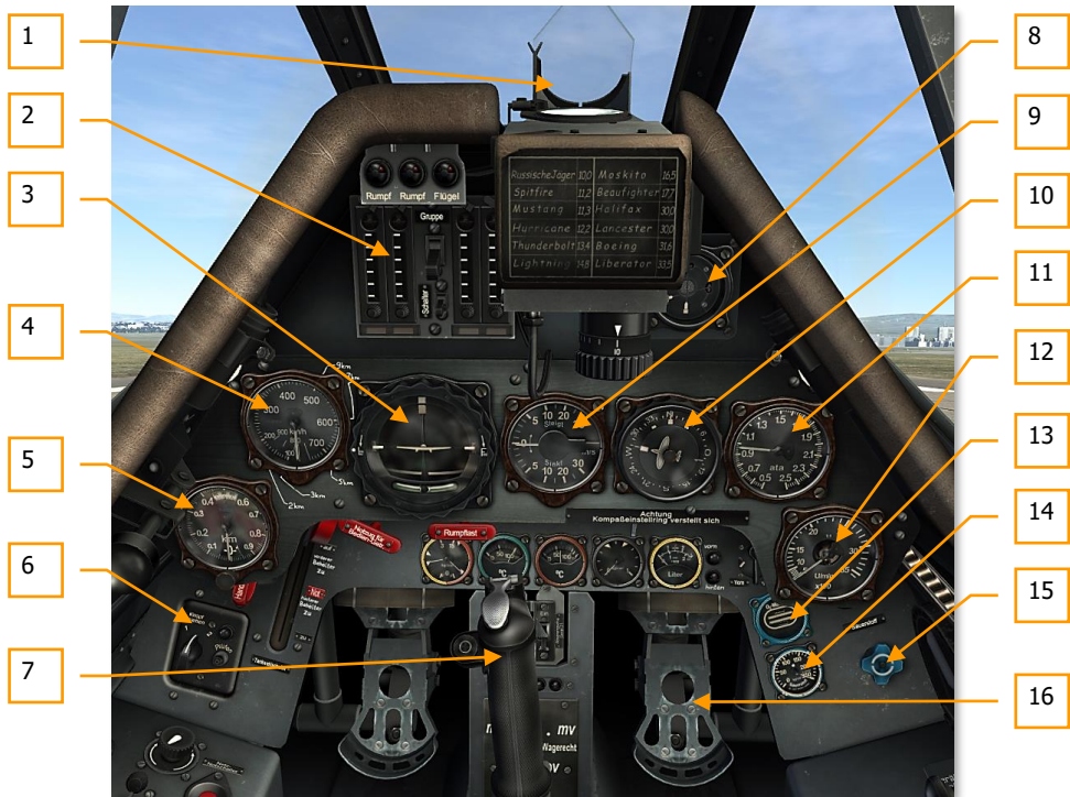
Figure 38: Fw 190 D-9 front dash
