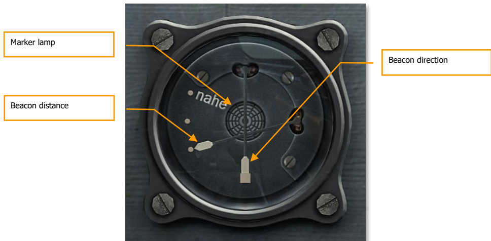
Figure 49: AFN-2 homing indicator
