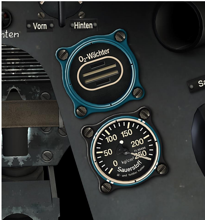
Figure 30: Oxygen flow indicator and pressure gauge
